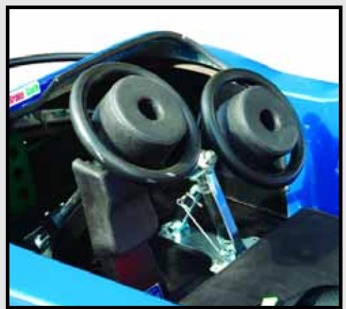
Optional mock steering wheel for the passenger is adjustable and removable.
